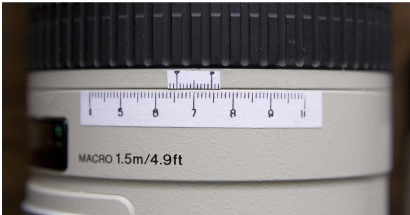
If you wish to try this, just print an appropriate sized version of the first figure for your needs and cut each scale out. You just need a length of the short one that covers two of the large index marks but it is convenient to have a longer section of the larger scale. I have attached the scales to my lens using paper glue. For weather resistance, the scales can be covered with clear tape.
